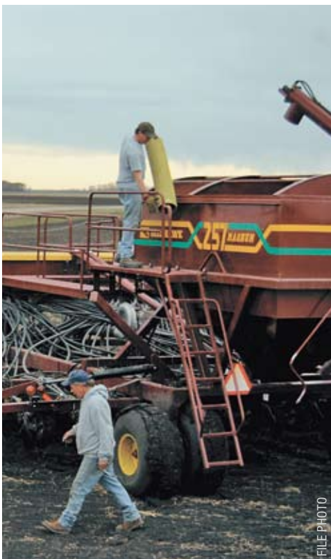
For best results, check implements frequently to ensure they are seeding at a proper and uniform depth.
