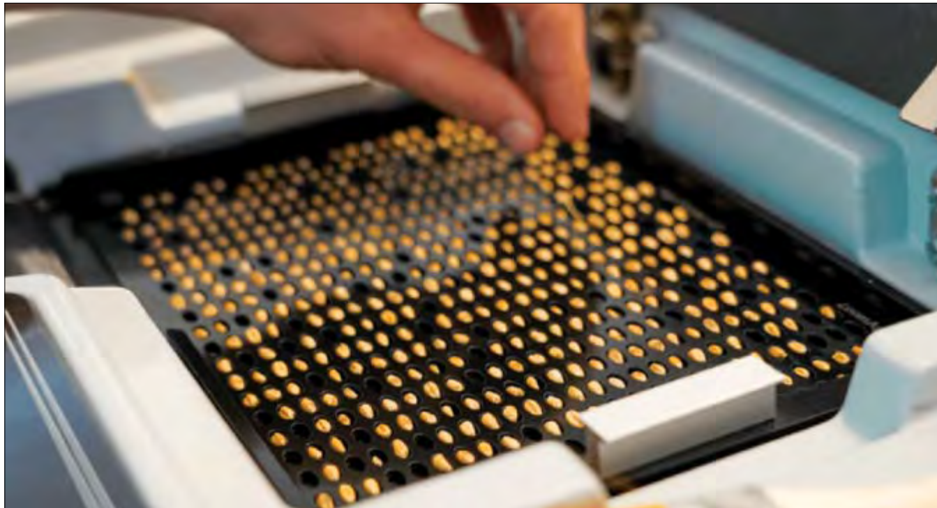
A special holder on the ZoomAgri machine keeps clean barley kernels separate in preparation for scanning. | ZOOMAGRI PHOTO
